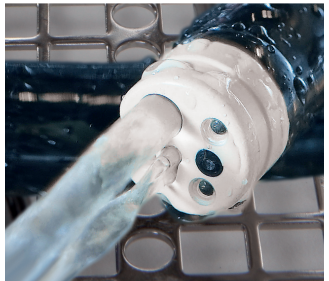
High cleaning performance: The endoscope channels are each individually cleaned, disinfected and dried.
