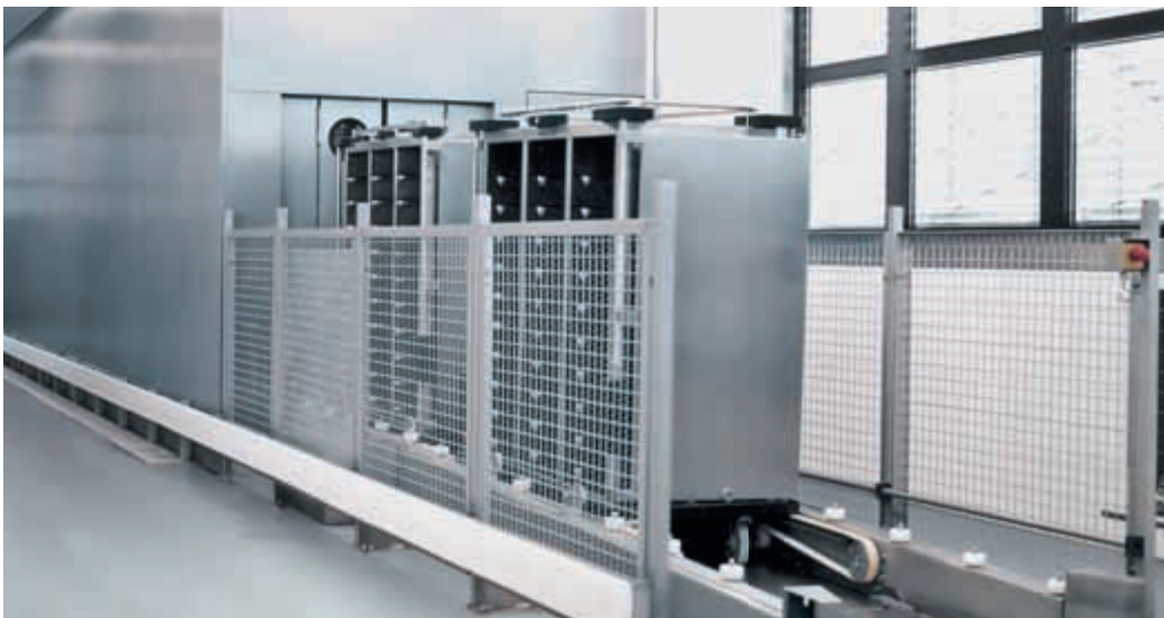
CLEANSTATION multichamber system with automatic loading and unloading Processes up to 60 transport carts/hour
