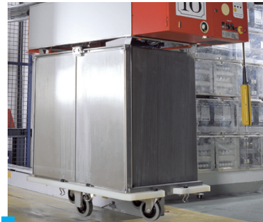
Automated trolley transport, suspended on the top-mounted electric conveyor
