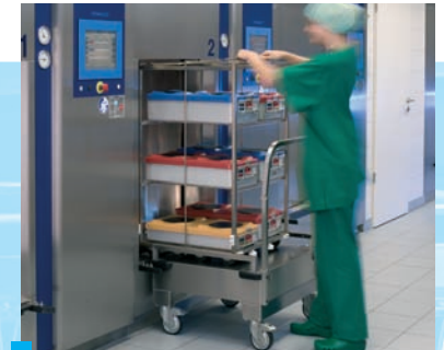
Transfer of the insert stand into the steriliser by direct docking
